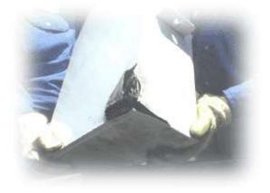
Figure 2 - Restrike Caused 5 Capacitors to Rupture Like the Opening of a Sardine Can as Shown Above
