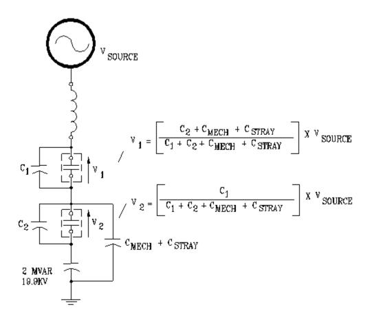
Figure 4 - Capacitor Voltage, Vacuum Bottle Voltage and Line Voltage With Cmech + Cstray =35Pf
