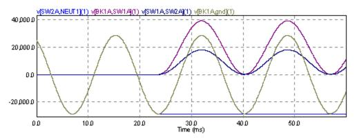
Figure 5 - Capacitor Voltage, Vacuum Bottle Voltage and Line Voltage With Cmech + Cstray =35Pf
