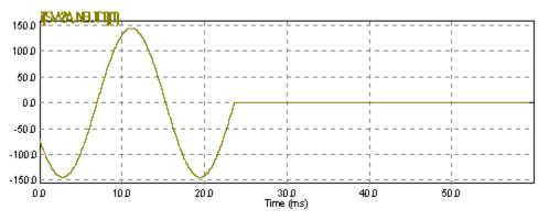
Figure 6 - Capacitor Current With Cmech + Cstray =35Pf
