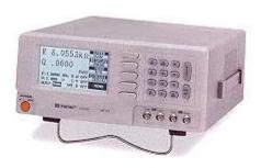
Figure 7 - A High Precision LCR Meter With an Accuracy On The Order of 0.05% in the Picofarad Range is Required to Ensure Equal Capacitance Accross the Vacuum Bottles
